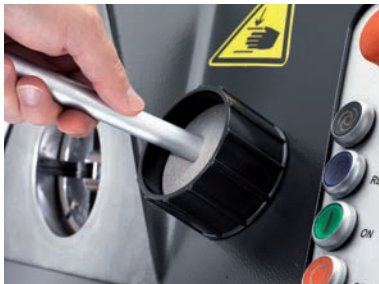
Oil sponge enables tube end to be moistened.
